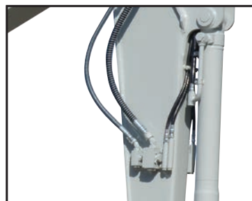
Auxiliary Hydraulic Lines
