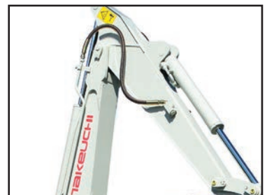
Auxiliary Hydraulic Lines
